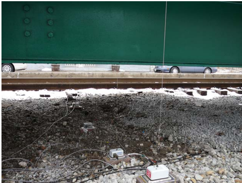
Figure 2. Cable Extension Transducers used to monitor deflections.
